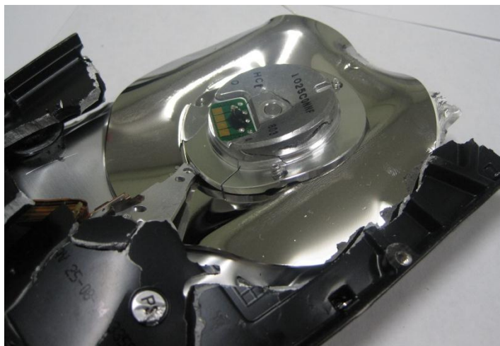
Platter Crushed, Warped and Mangled by Phiston MediaVise's Interlocking Plates
